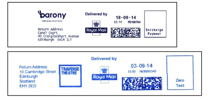
Finally for this section, Duncan sends this printing error seen on a Francotyp-Postalia PostBase machine, where a ghost '2' is shown in the upper part of the indicia block. It seems that the item was misfed as it entered the machine because the frank starts on the extreme right hand side of the envelope and this may, in turn, have caused the printing 'hiccup'. Note that the lower printer has failed as well because the words 'Address' and 'Blackpool' also contain double-printed letters.
